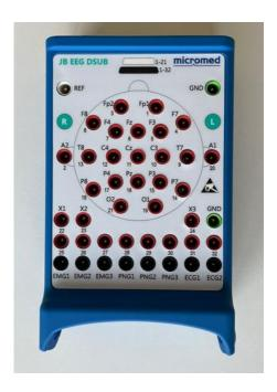
The **JB EEG DSUB** jackbox has the same size and shape oft he existing **JB TOPHAT** and can be used in combination with the following 32 channel head boxes:
